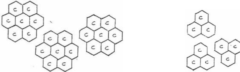
If the moisture content of London Clay is increased to approximately 55%, the London Clay particles have even more water around them (see below left). The subsoil volume has increased again and decreased in density. If the moisture content of London Clay is decreased from 55% to 25%, the subsoil decreases in volume significantly (see below right).
