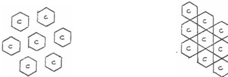
Two-dimensionally, a reduction in moisture content from 32% to 25% represents approximately a 7% reduction in subsoil volume. Whereas, a reduction in moisture content from 55% to 25% represents over a 30% reduction in subsoil volume. I believe this degree of subsoil shrinkage would have dramatic results.
